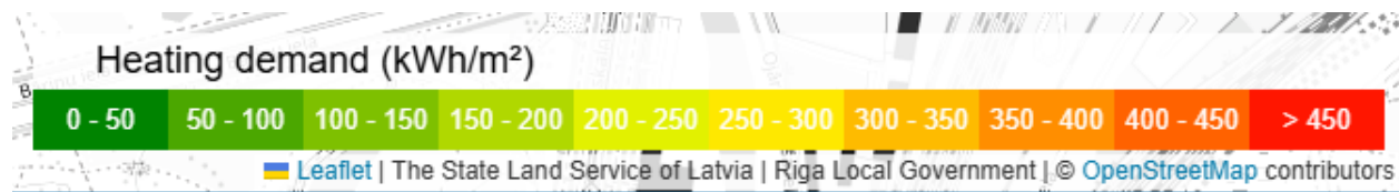
Figure 7. EPC-based colour scale for heating energy demand
